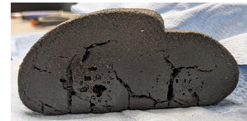
MW sintered RDW simulant (bottom right) has semi-circular cracks around hot spot while other MW sintered simulants do not
