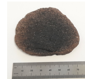
MW sintered RDW simulant (bottom right) has semi-circular cracks around hot spot while other MW sintered simulants do not
