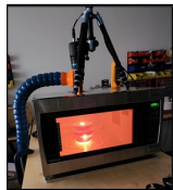
Ambient COTS microwave sintering of JSC-1A simulant
