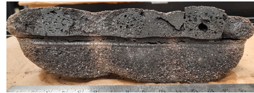
MW sintered RDW simulant (bottom right) has semi-circular cracks around hot spot while other MW sintered simulants do not
